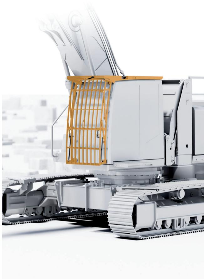
For work where no FOPS is required, the front guard can be removed from the main field of view using the gas pressure spring-assisted swivelling mechanism. This enables a clear view within a few seconds for nonhazardous work.
